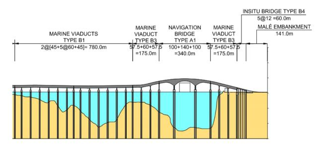
**Villingili-Gulhifalhu Link:** Between Villingili and Gulhifalhu islands where water depth deepens sharply toward the center of the channel, another 140m-span balanced cantilever box girder bridge is proposed. The mainline of the bridge will continue as marine viaducts along the shoreline of Villingili (right hand side of figure below). An interchange and connecting ramps to Villingili Island is proposed that requires some reclamation.
